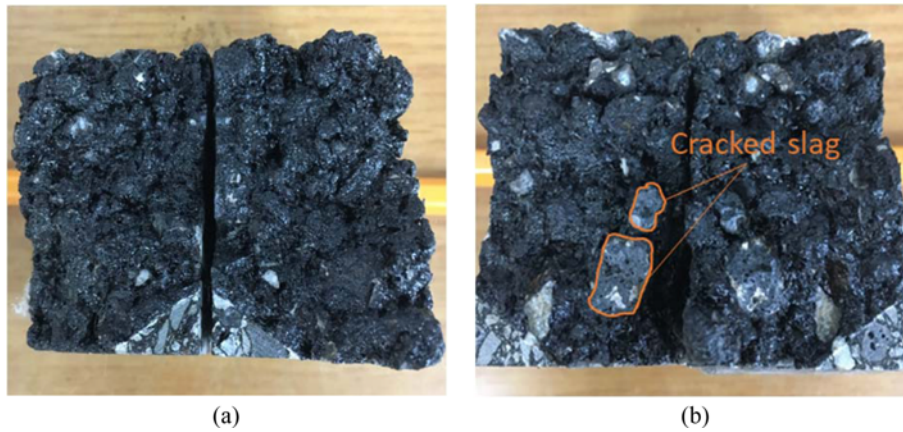
Fig. 10. The Cracking Surface of: (a) NF Specimen, (b) SF Specimen
