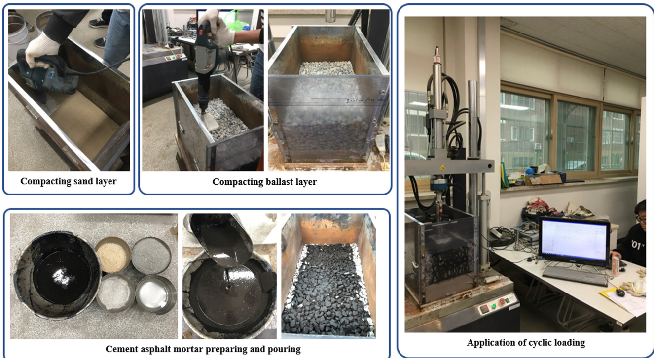
Fig. 4. Mockup test set up showing: a) sand layer compacting, b) ballast layer compacting, c) CAM mixing and pouring, d) cyclic loads application.
