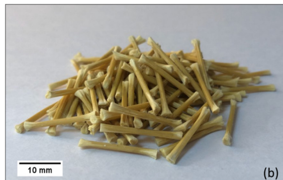
Fig. 8. Diameter of WMA coated fiber (a), morphology of WMA coated fiber (b).
