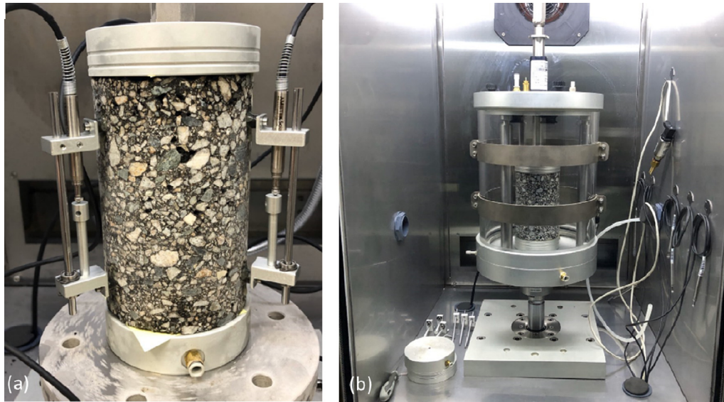
Fig. 6. Dynamic modulus test (a) and unconfined flow number test (b).
