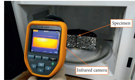
FIGURE 4: Microwave heating test setup.
