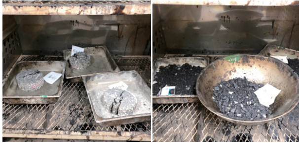
Fig. 3 The damaged samples from indirect tensile strength test were loosed mix at 150 °C for 6 hours.
