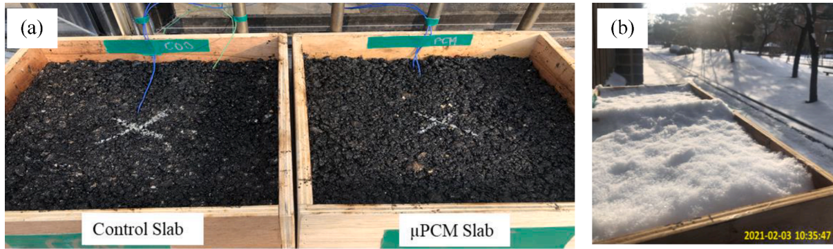
Fig. 6. (a) Outdoor temperature test set up, (b) temperature recording on snow day.
