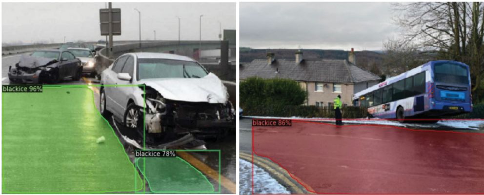
Figure 14. Black ice detection results of the trained model.
