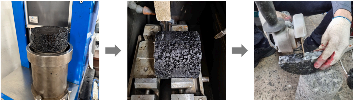
Fig. 4. Semi-circular bending sample preparation.
