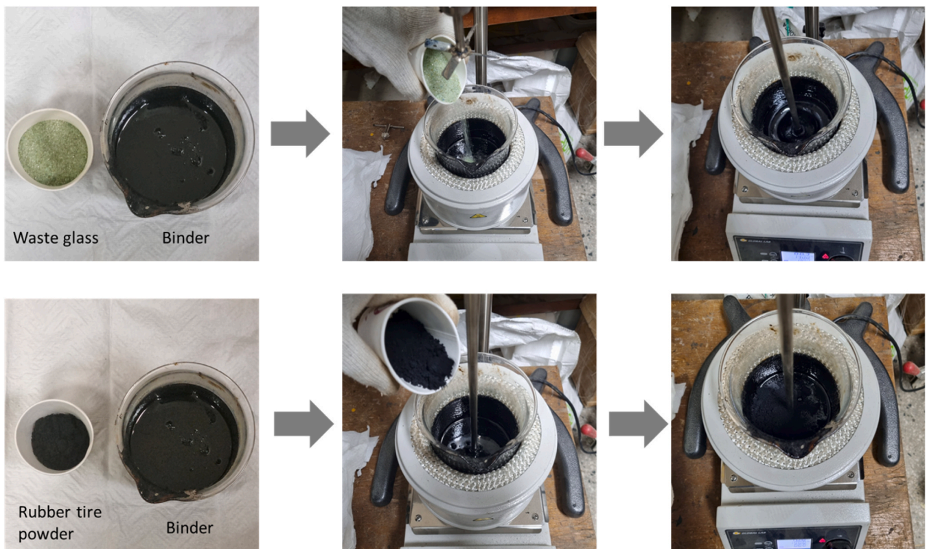
Fig. 1. Asphalt binder mixing process.
