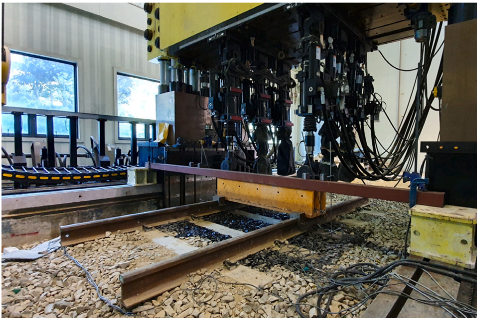
Fig. 3. Construction of Testbed and Measurement Instruments setup.
